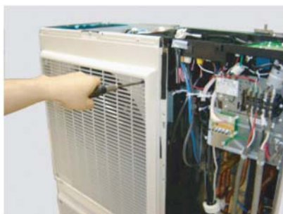
Remove the 4 mounting screws.
