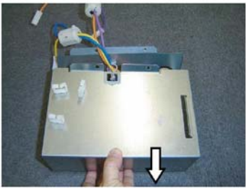
Remove the CONDENSER COVER by sliding toward.
