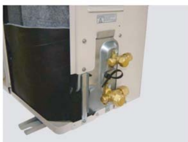
Remove the VALVE COVER.
